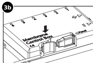
**3b** Squeeze the cable into the strain relief hook on the box as illustrated.
