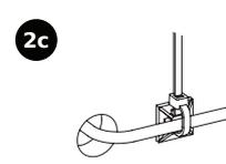
**2c** Attach the cable using the cable tie\* and hook onto the wall to avoid accidental drop of the cable.
