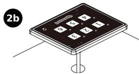
**2b** Mount the panel firmly onto the dashboard with self-adhesive in the back.
