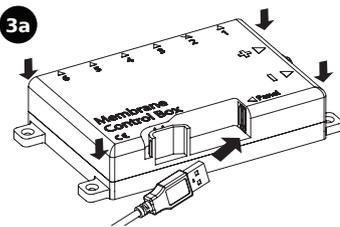
**3a** Install the control box properly with the screws\*. Insert the other end of the **micro USB** cable into the control box.
