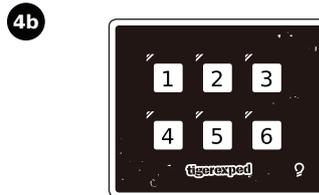
**4b** Connect the load terminals to the desired devices. The numbers on top of the load terminals correspond to the numbers on the membrane touch panel as shown in the left.
