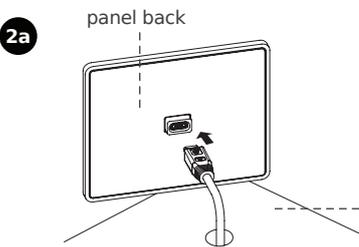
**2a** From the back of dashboard, insert the **micro USB cable\*** to the front. Connect the micro USB plug to the socket to the back of panel.
