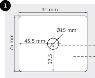
**1** Mark the hole at the desired panel position on your dashboard and cut the hole accordingly.
