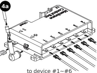
**4a** Crimp the **DC positive wire (+)** with the round terminal\*. Pass the wire through the insulator\* and connect to the screw terminals. Cover the terminals with the insulator properly. Crimp the **DC negative wire (-)** with the insulated 0.250" female terminal and insert into the negative quick terminal\* on control box.
