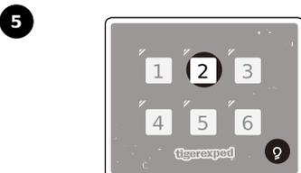
**Momentary Button Set-up** To set up a specific button to be momentary (Push-On), press the button and the backlight button simultaneously for more than 5 seconds until the button blinks.
