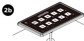
**Mount the panel** firmly onto the dashboard with self-adhesive in the back.
